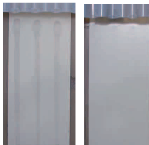
一般のコラー鋼板 Conventional pre-painted steel 耐汚染性カラー鋼板 New type of pre-painted steel
